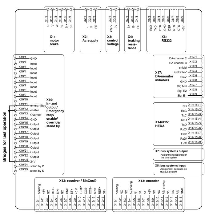
The assignment of X12 does not apply for the S3 option.
